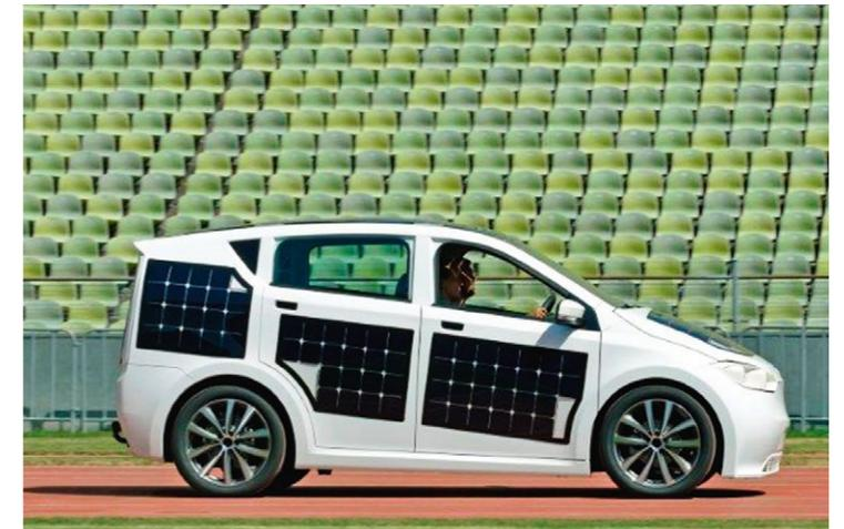
photovoltaic (PV) cells directly integrated into its bodywork. The car can also be recharged in a more "conventional" way. Either in rapid mode, via charging points that are compatible with other electric vehicles, or in slow mode, by connecting the car to a household power outlet for 8 hours.
