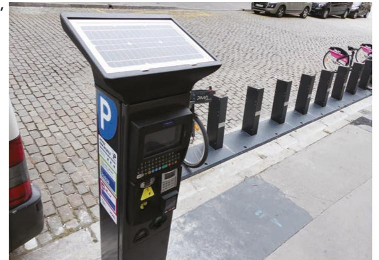
**Topped with solar cells, the parking meters are self-operated and don't need to be connected to the grid.**
