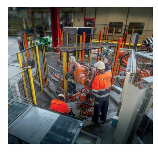
Retrofitting involves refurbishing all the internal components of a machine in order to increase its reliability and bring it up to date. In the current economic and environmental climate,
